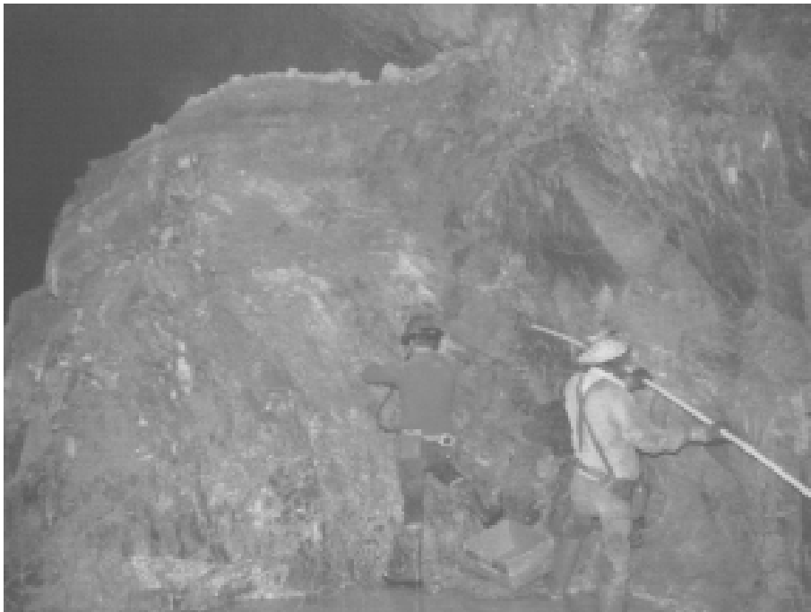
Loading a slash round in jointed and decomposed pegmatite
