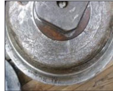
wear at housing
