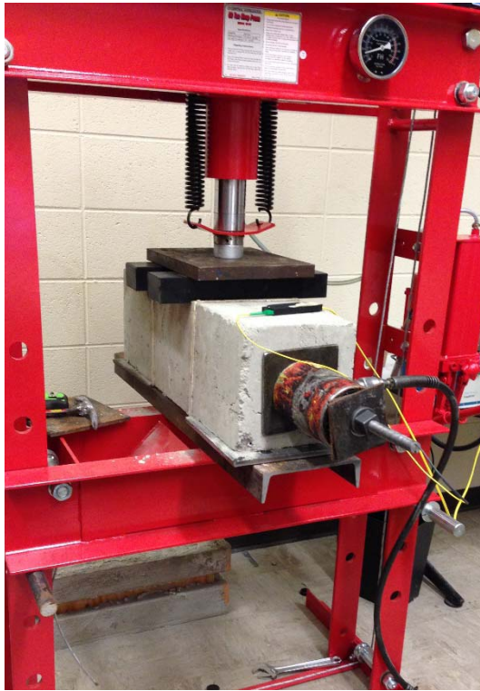
Embedded rebar specimen
