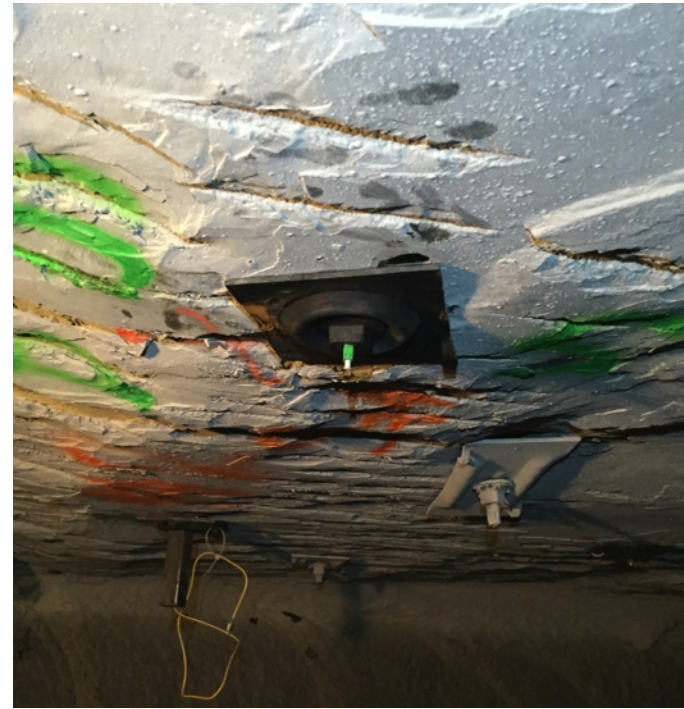
3-groove DOS instrumented bolt installed in shale roof of a coal mine
