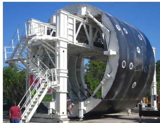
Figure 4. Tunnel form inspection.
