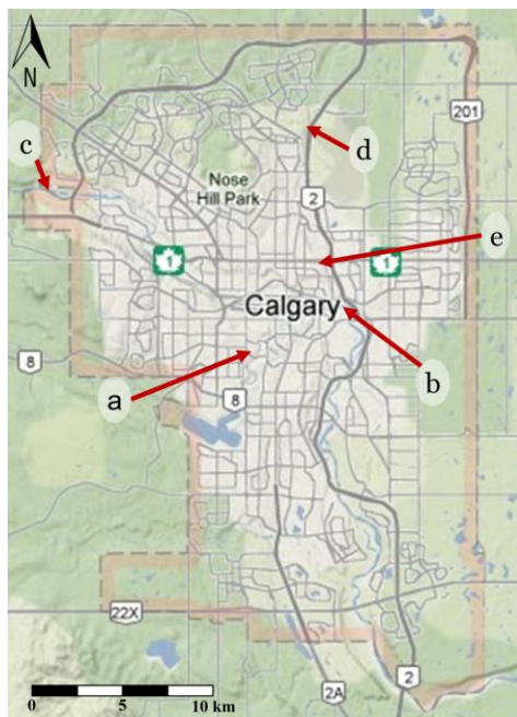
Figure 7: TBM project locations in Calgary AB; a) Glencoe Storm Sewer Upgrade, b) 15 th Street Syphon Upgrade, c) Valley Ridge Feedermain, d) Beddington South Sanitary Upgrade, e) Nose Creek Sanitary Trunk Upgrade. (Google, 2012)
