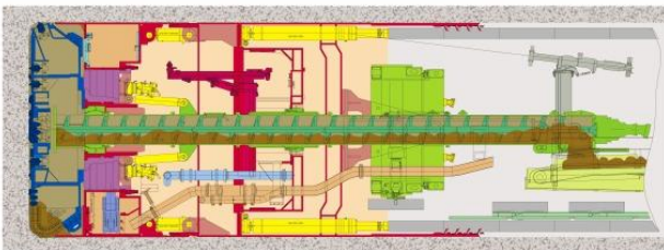
Figure 6. TBM Operation open mode
