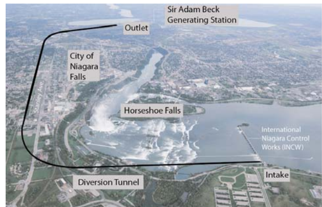
Figure 1. Original Route of the new Niagara Tunnel
