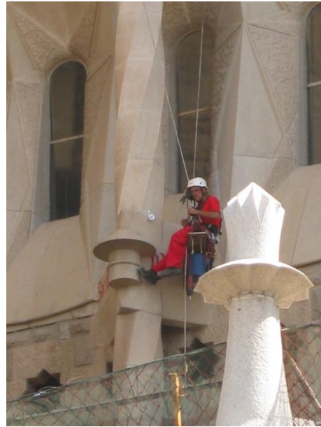
Figure 9. Monitoring of the displacements inside the Temple (robotic theodolite on the left and target placement on the right)
