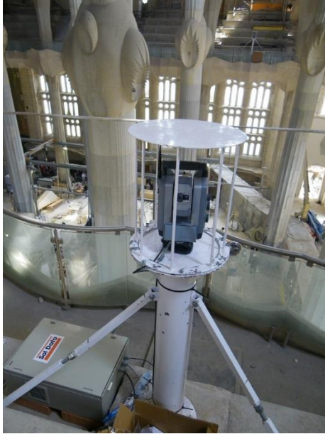
Figure 9. Monitoring of the displacements inside the Temple (robotic theodolite on the left and target placement on the right)
